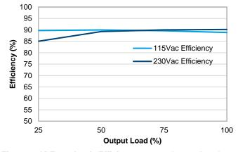
Fig. 1-1. ADT-060A12A Efficiency versus Output Load
