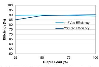
Fig. 1-3. ADT-060A19A Efficiency versus Output Load
