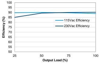
Fig. 1-4. ADT-060A24A Efficiency versus Output Load
