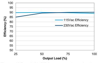
Fig. 1-2. ADT-060A15A Efficiency versus Output Load
