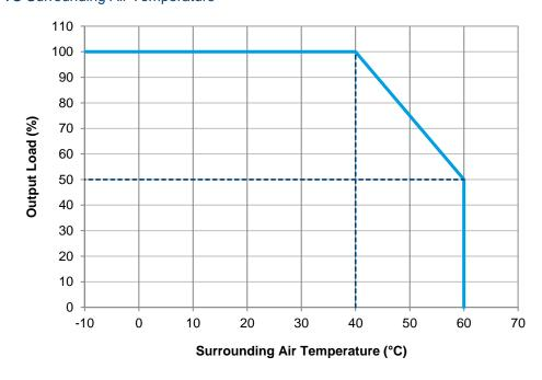
Fig. 2 De-rating for All Mounting Orientation (All Models) > 40°C de-rate power by 2.5% / °C
