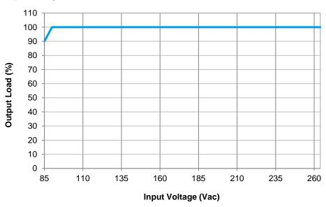
Fig. 3 De-rating for Low Input Voltage (All Models) < 90 Vac de-rate power by 2% / Vac
