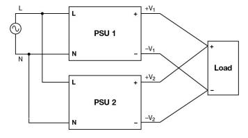
Fig. 4 Parallel Operation Connection Diagram
