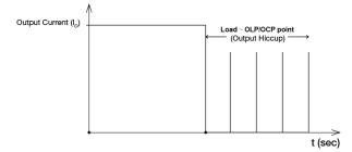
It is not recommended to prolong the duration of  $I_{\rm O}$  when it is less than OLP/OCP point, but greater than 100%, since it may cause damage to the PSU.
