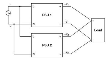
Fig. 4 Parallel Operation Connection Diagram
