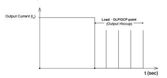
It is not recommended to prolong the duration of  $I_0$  when it is less than OLP/OCP point, but greater than 100%, since it may cause damage to the PSU.
