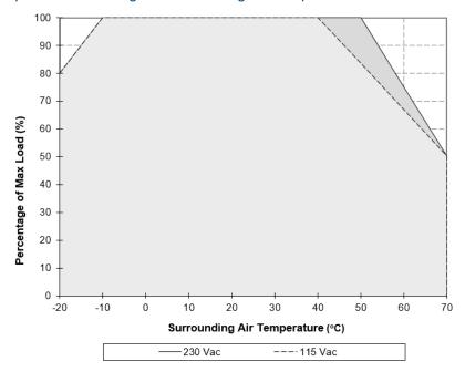
Fig. 1 De-rating for Vertical Mounting Orientation
