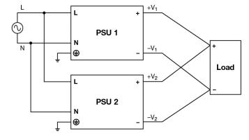
Fig. 4 Parallel Operation Connection Diagram
