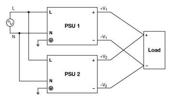
Fig. 4 Parallel Operation Connection Diagram
