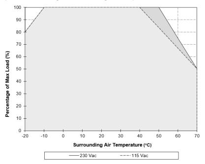
Fig. 1 De-rating for Vertical Mounting Orientation
