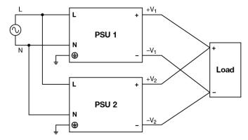
Fig. 4 Parallel Operation Connection Diagram
