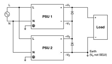
Fig. 11 Series Operation Connection Diagram
