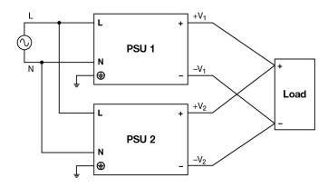
Fig. 10 Parallel Operation Connection Diagram
