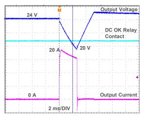
Fig. 8.2 APB 400% of nominal output current for 2 ms
