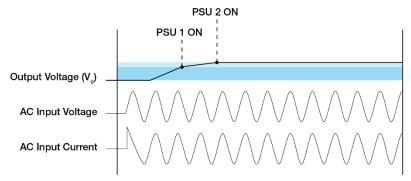
The turn ON would be non-monotonic as the power supply with the fastest startup time and rise time will turn on first. As a result, the startup waveform with 2 power supplies connected in series would see a step.
