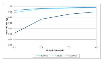
Fig. 4 Power Factor Vs Output Load at 24 V
