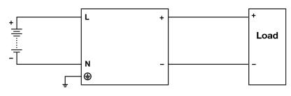
Fig. 12 DC Input Operation Connection Diagram
