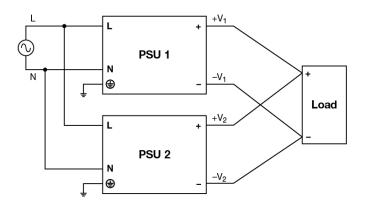
Fig. 10 Parallel Operation Connection Diagram
