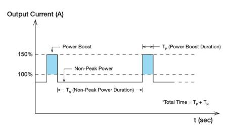
Fig. 7 Duty Cycle Calculation
