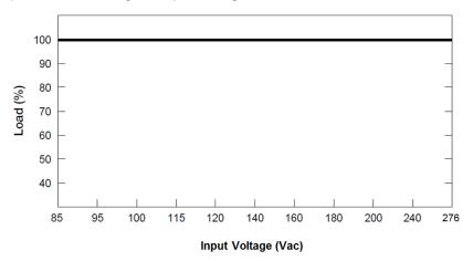
No output power de-rating for the input voltage range
