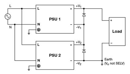
Fig. 11 Series Operation Connection Diagram
