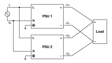
Fig. 10 Parallel Operation Connection Diagram
