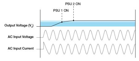
The turn ON would be non-monotonic as the power supply with the fastest startup time and rise time will turn on first. As a result, the combined output voltage waveform of the 2 power supplies connected in series will include a step.
