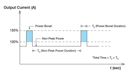
Fig. 7 Duty Cycle Calculation
