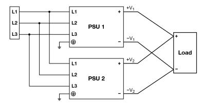
Fig. 10 Parallel Operation Connection Diagram
