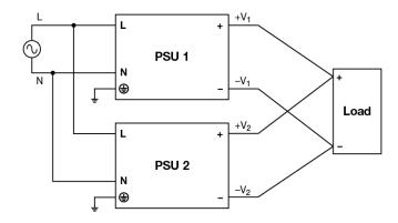
Fig. 6 Parallel Operation Connection Diagram
