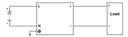
Fig. 8 DC Input Operation Connection Diagram
