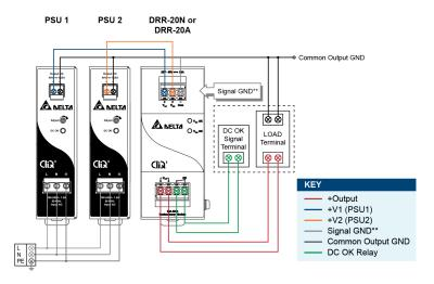
\*\*The Signal GND in the DRR module is for the built-in LED and DC OK signals. The Output GND terminals from the two PSU's do not need to be connected to the Signal GND terminal.
