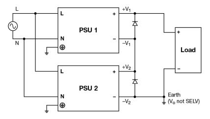
Fig. 7 Series Operation Connection Diagram
