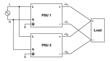
Fig. 6 Parallel Operation Connection Diagram
