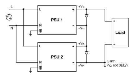
Fig. 7 Series Operation Connection Diagram
