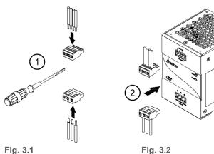
**CAUTION:** Must tighten wire to housing (Fig. 3.1) before plugging into the terminal block connection (Fig. 3.2).
