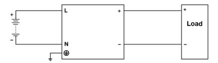
Fig. 8 DC Input Operation Connection Diagram
