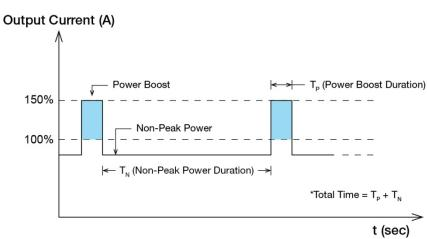
Fig. 4 Duty Cycle Calculation
