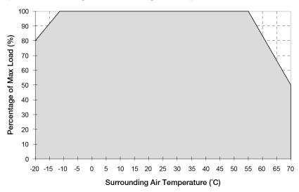
Fig. 1 De-rating for Vertical Mounting Orientation
