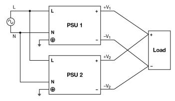
Fig. 4 Parallel Operation Connection Diagram
