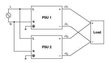
Fig. 4 Parallel Operation Connection Diagram
