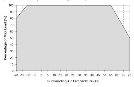
Fig. 1 De-rating for Vertical Mounting Orientation
