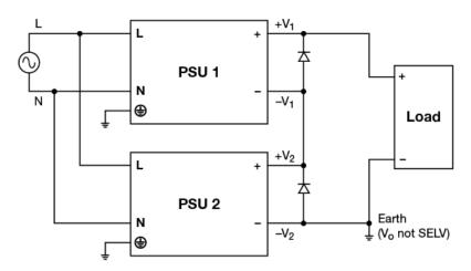
Fig. 11 Series Operation Connection Diagram
