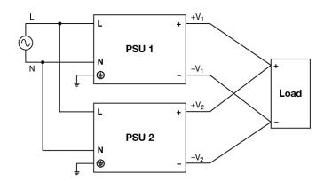
Fig. 10 Parallel Operation Connection Diagram
