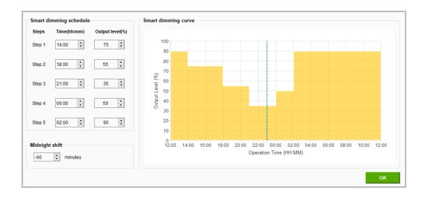
**Ratio Rescale Timer**: This mode is similar to Midnight Centric Timer that records the power-on time based on the local night time. The Ratio Rescale Timer software rescale programmed output power profile of each step by a calculated percentage of the recorded power-on time out of given 5 steps duration.
