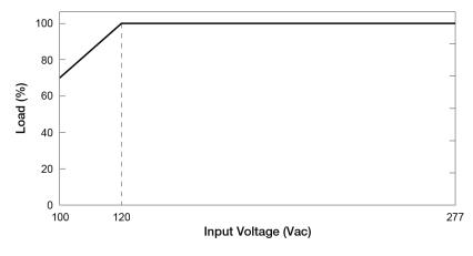
■ No output power de-rating for the input voltage from: 120Vac to 277Vac
