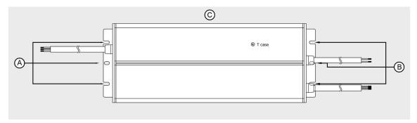
Fig. 3 Mounting Hole Locations
