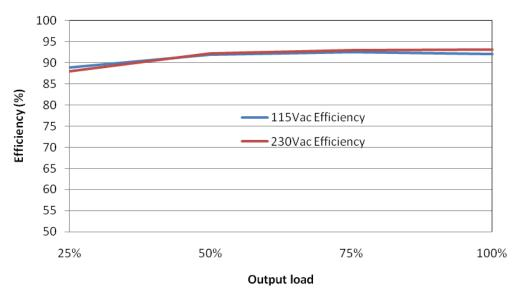
Fig.1 Efficiency versus output load
