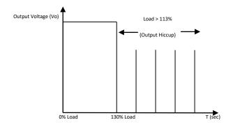
Additionally, if the  $I_{\rm O}$  is <130% but >110% for a prolong period of time (depending on the load), the Over Temperature Protection (OTP) will be activated due to high temperature on critical components. The power supply will then go into hiccup mode until the fault is removed; and, the input voltage is removed, then reapplied.
