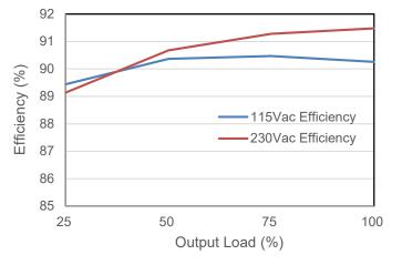
Figure 1-3 MEA-065A19C Efficiency versus Output Load
