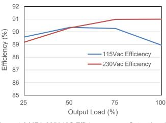
Figure 1-2 MEA-065A15C Efficiency versus Output Load
