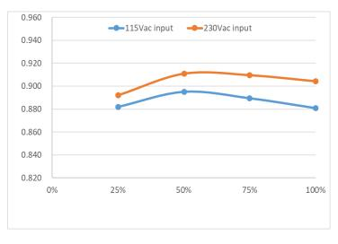
Figure 1. Typical efficiency Curve for 12 V (exclude fan power)
