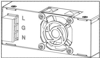
American Barrier Strip Conductor size: AWG 20 to 14. Tightening torque:8 kgf.cm.
