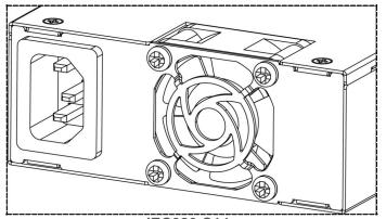
IEC320 C14 Conductor size: AWG 20 to 14 Mating with IEC320 C13
