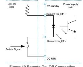
Figure 10 Remote On\_Off Connection
