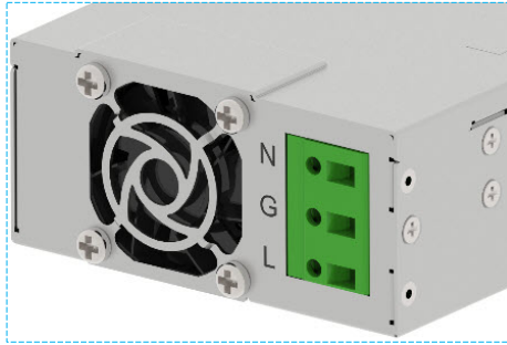
Figure 5. European Terminal Block TIGHTENING TORQUE:2.4 Lbf.in
