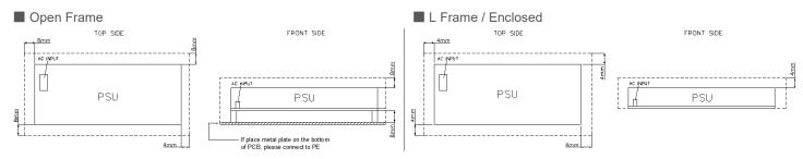
For safety reasons, please ensure the mounted device is kept safety distance as below at all sides from other components and equipments. a) For Open Frame Type  $\geq$  8 mm (0.315 inch) from primary side and  $\geq$  4 mm (0.16 inch) from secondary side. b) For with Case Type  $\geq$  4 mm (0.16 inch)
