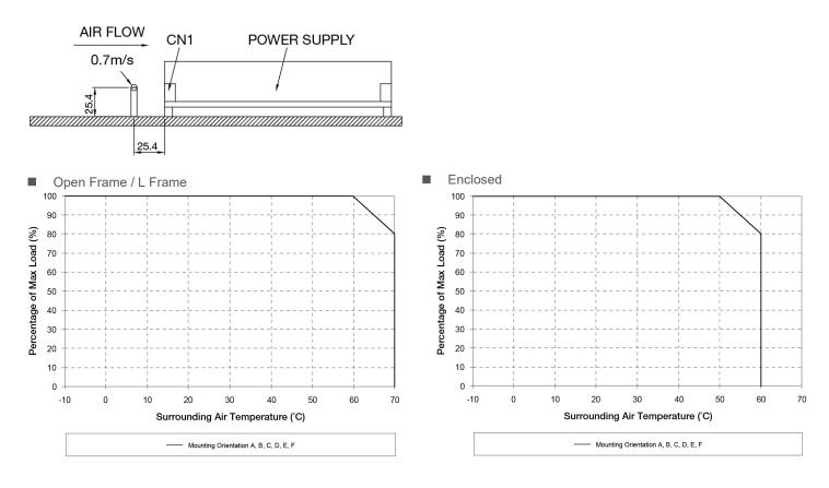
Fig.1.3 De-rating for Mounting Orientation A to F > 60°C de-rate power by 2% / °C
