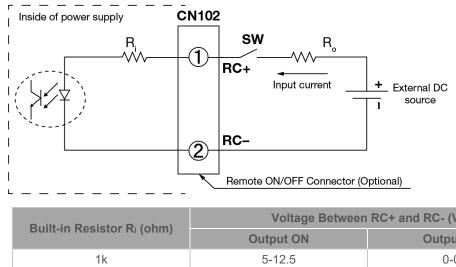
You can remotely control the power supply unit to turn ON/OFF by using an external DC source. Follow the DC power source voltage and current limiting defined in the table below.
