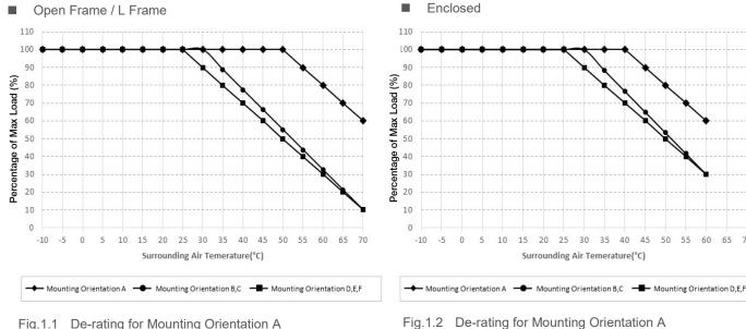
Fig.1.1 De-rating for Mounting Orientation A > 50°C de-rate power by 2% / °C De-rating for Mounting Orientation B, C > 30°C de-rate power by 2.25% / °C De-rating for Mounting Orientation D, E, F > 25°C de-rate power by 2% / °C
