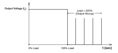
It is not recommended to prolong the duration of  $I_{\rm O}$  when it is <220% but >100%, since it may cause damage to the PSU.
