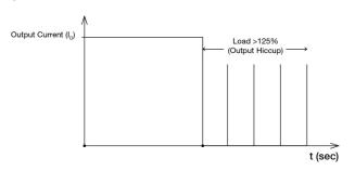
It is not recommended to prolong the duration of I<sub>O</sub> when it is <125% but >100%, since it may cause damage to the PSU.
