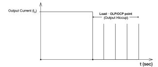
It is not recommended to prolong the duration of I<sub>0</sub> when it is less than OLP/OCP point, but greater than 100%, since such an overload condition may cause damage to the PSU.
