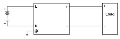
Fig. 5 DC Input Operation Connection Diagram
