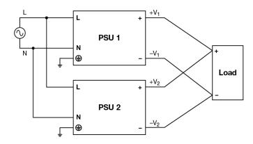
Fig. 4 Parallel Operation Connection Diagram
