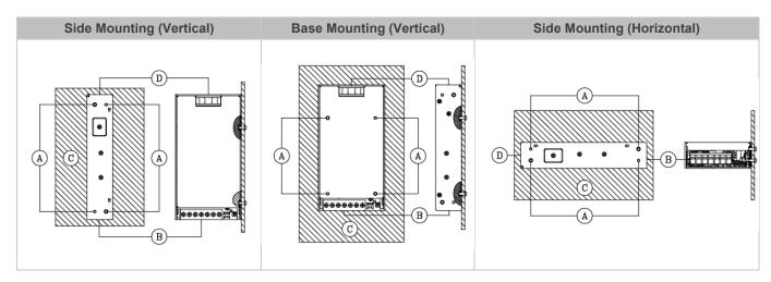
Fig. 2 Mounting Orientation
