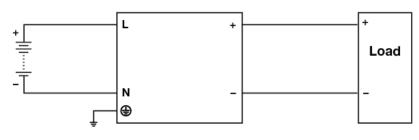
Fig. 5 DC Input Operation Connection Diagram
