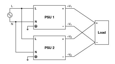
Fig. 4 Parallel Operation Connection Diagram
