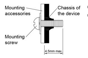
Only use M4 screw ≤ 4.5 mm through the base mounting holes. This is to keep a safety distance between the screw and internal components.
