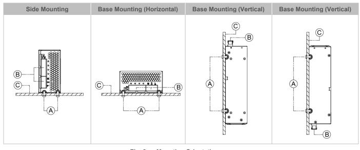
Fig. 2 Mounting Orientation
