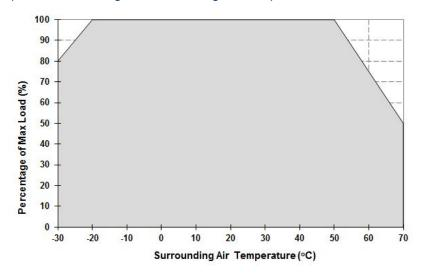
Fig. 1 De-rating for Vertical and Horizontal Mounting Orientation -20°C to -30°C de-rate power by 2.0% / °C > 50°C de-rate power by 2.5% / °C
