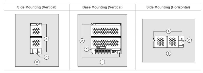
Fig. 2 Mounting Orientation
