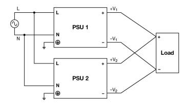
Fig. 4 Parallel Operation Connection Diagram
