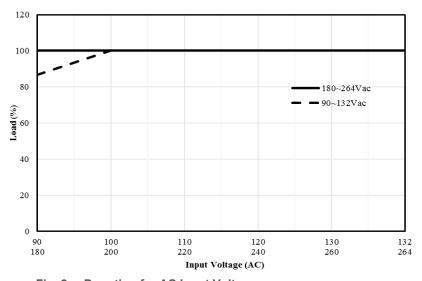
Fig. 2 De-rating for AC Input Voltage < 100 Vac de-rate power by 1.33% / V
