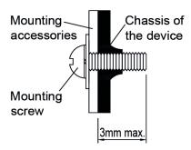
Fig. 4 Mounting Screw
