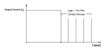
It is not recommended to prolong the duration of lo when it is <110% but >100%, since it may cause damage to the PSU.
